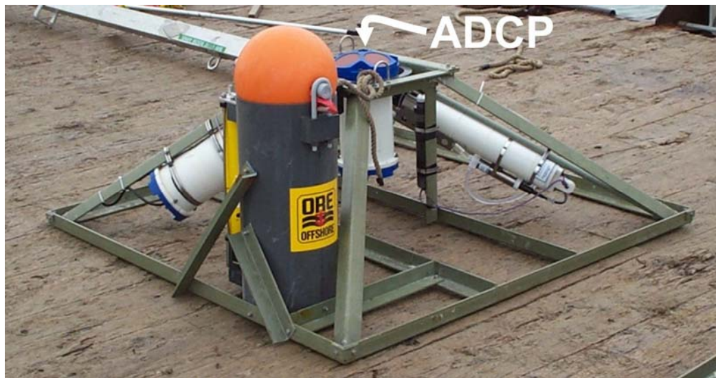
Figure 6. An example of the oceanographic mooring employed for our measurements. The top of the ADCP is approximately 0.5 m above the frame bottom. The orange pop-up buoy facilitates recovery at the end of the deployment. The fat white pressure case on the left contains extra battery power for the ADCP; the thin white pressure case on the right is an instrument that measures pressure, temperature, salinity and transmissivity.
