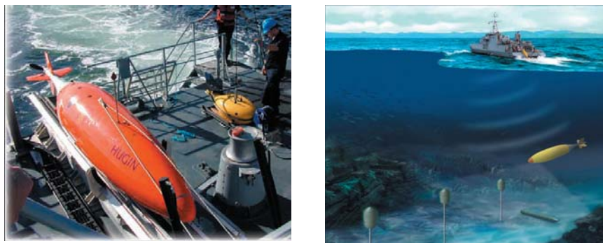
Figure 14. The Hugin AUV, manufactured by Kongsberg Maritime. This AUV has an endurance of up to one day, can dive to 1000 m depths and can travel at over 4 knots.
